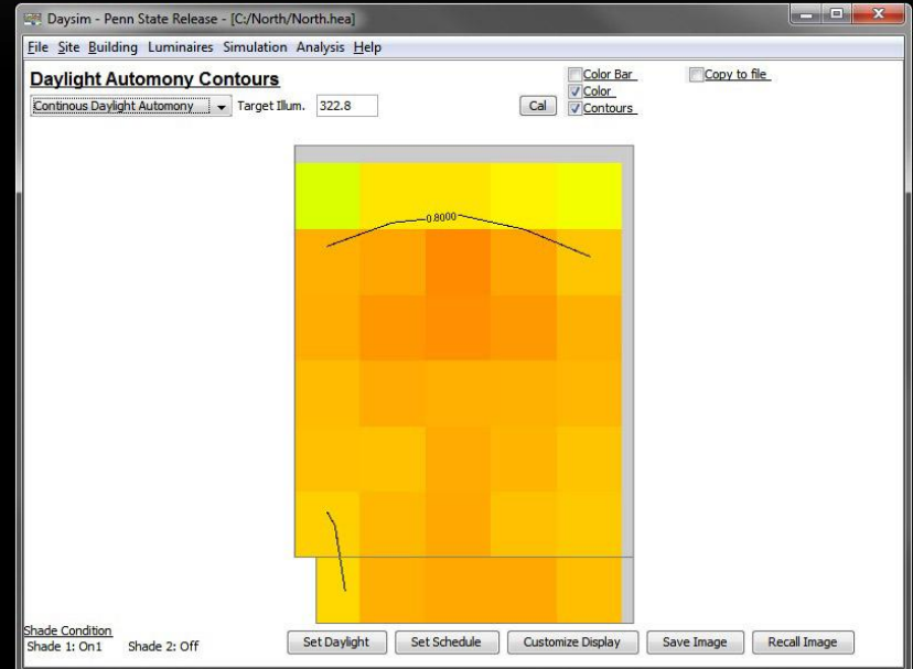
Continuous Daylight Autonomy
